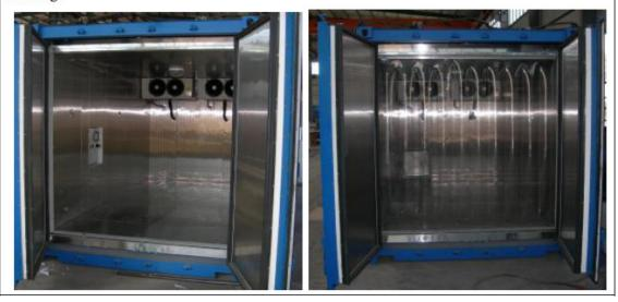
The main frame strength members and corner fittings of the container are constructed of welded steel parts, which are protected against corrosion by hot dip galvanizing. The walls and the roof is made of 100mm PU glass reinforced plastic insulation panel for internal and external surfaces and cover the internal surface with stainless steel plates to avoid corrosion and water leakage. The floor is made of corrugated stainless steel plate.
